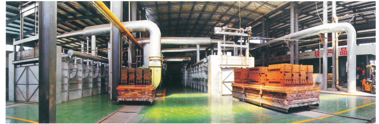
环保节能超高温隧道窑 Environmental protection and Energy saving ultra-high temperature tunnel kiln
